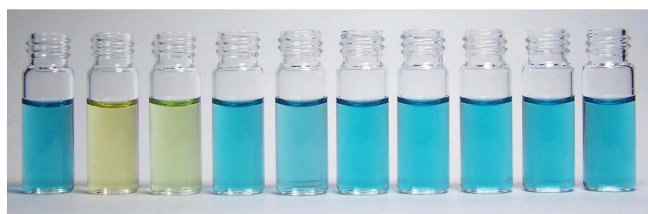
Figure 10. Color shown by [\text{Zn}_2(\mathbf{1})(\mathbf{2})]^{2+} ( 25 \mu\text{M} ) in the absence and presence of anions ( 25 \mu\text{M} ). From left to right: no anion, ATP, ADP, AMP, \text{HPO}_4^{2-} , \text{SO}_4^{2-} , \text{CH}_3\text{CO}_2^- , \text{HCO}_3^- , \text{Cl}^- , and \text{NO}_3^- .
