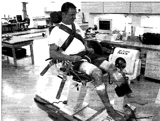
Fig. 2. Isokinetic test using Biodex system.
