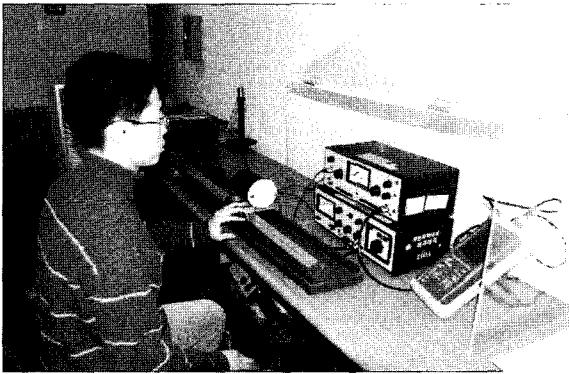
Fig. 1 Measurement of absorption coefficient by impedance tubes
