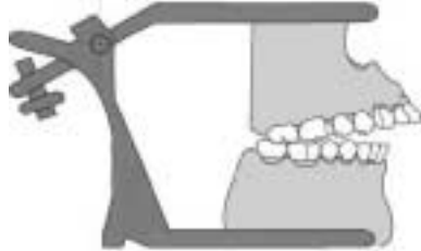
Fig. 11. Simple hinge articulator mounted posterior THA deviation(Type b).
