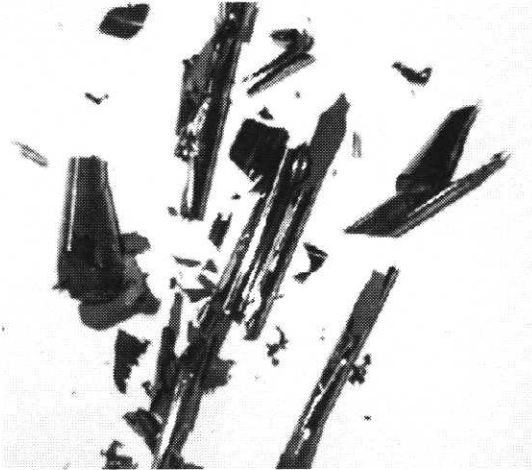
Fig. 6. Formed pyrocarbon film on the reactor wall.
