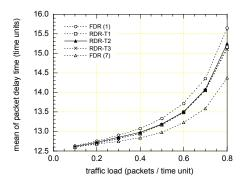
Fig. 3. Mean of packet delay time with respect to traffic load (duplication rules: FDR, RDR-T1, RDR-T2, and RDR-T3, W=100, L=8,  $\lambda \in \{0.1, \cdots, 0.8\}$ ,  $\varepsilon=0.001$ ) 그림 3. 트래픽 부하에 따른 평균 패킷 지연 시간 (중복 규칙: FDR, RDR-T1, RDR-T2, and RDR-T3, W=100, L=8,  $\lambda \in \{0.1, \cdots, 0.8\}$ ,  $\varepsilon=0.001$ )
