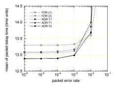
Fig. 4. Mean of packet delay time with respect to packet error rate (duplication rules: FDR, RDR-T1, ADR-T1, and ADR-T2, W=100, L=8,  $\lambda=0.5$ ,  $\varepsilon \in \{10^{-6}, \cdots, 10^{-1}\})$ 그림 4. 패킷 오류율에 따른 평균 패킷 지연 시간 (중복 규칙: FDR, RDR-T1, ADR-T1, and ADR-T2, W=100, L=8,  $\lambda=0.5$ ,  $\varepsilon \in \{10^{-6}, \cdots, 10^{-1}\})$
