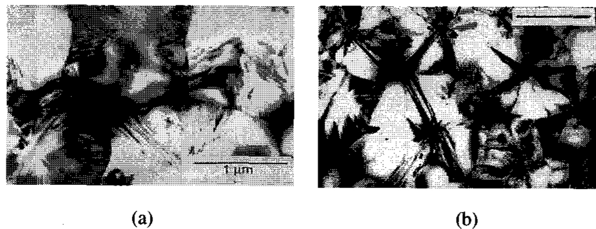
Fig. 2. Planar-view TEM images of Super-Lateral Growth (SLG) poly-Si for (a) LPCVD and (b) Ion-implanted LPCVD. Laser energy density is set to be the same for both cases. [Ref: 1,2]
