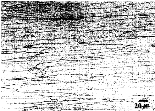
Fig. 2. Optical microstructure of unidirectionally solidified cast rod.
