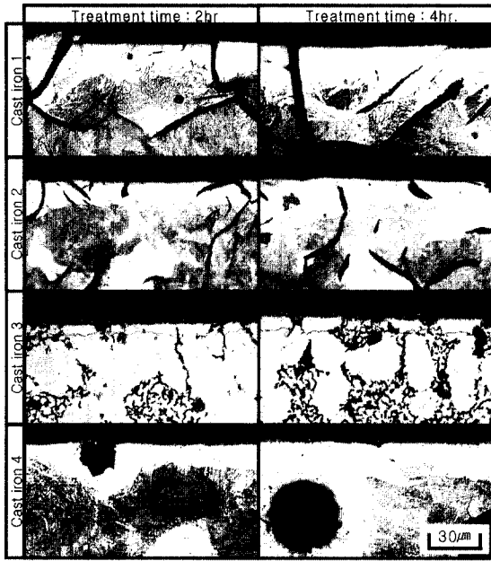
Fig. 2. Optical micrographs of cross-sections showing the effect of treatment time on the thickness of compound layer.
