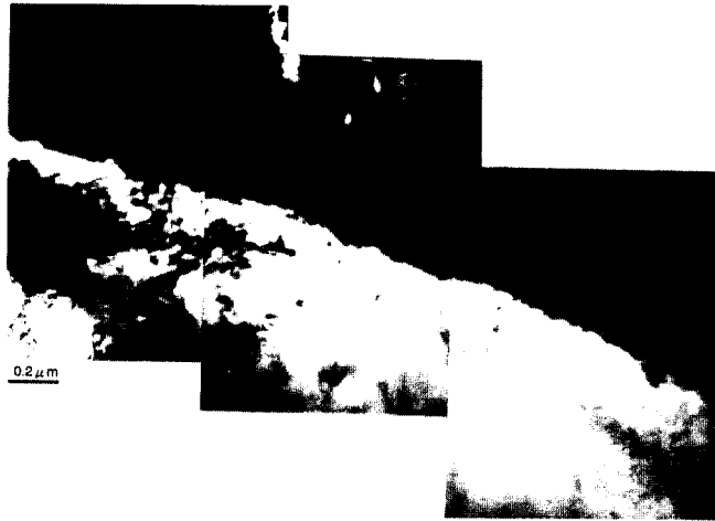
Fig. 2. The microstructure of the bonded interface of upset welding (Fe-sintered material and AC4C) observed by TEM.
