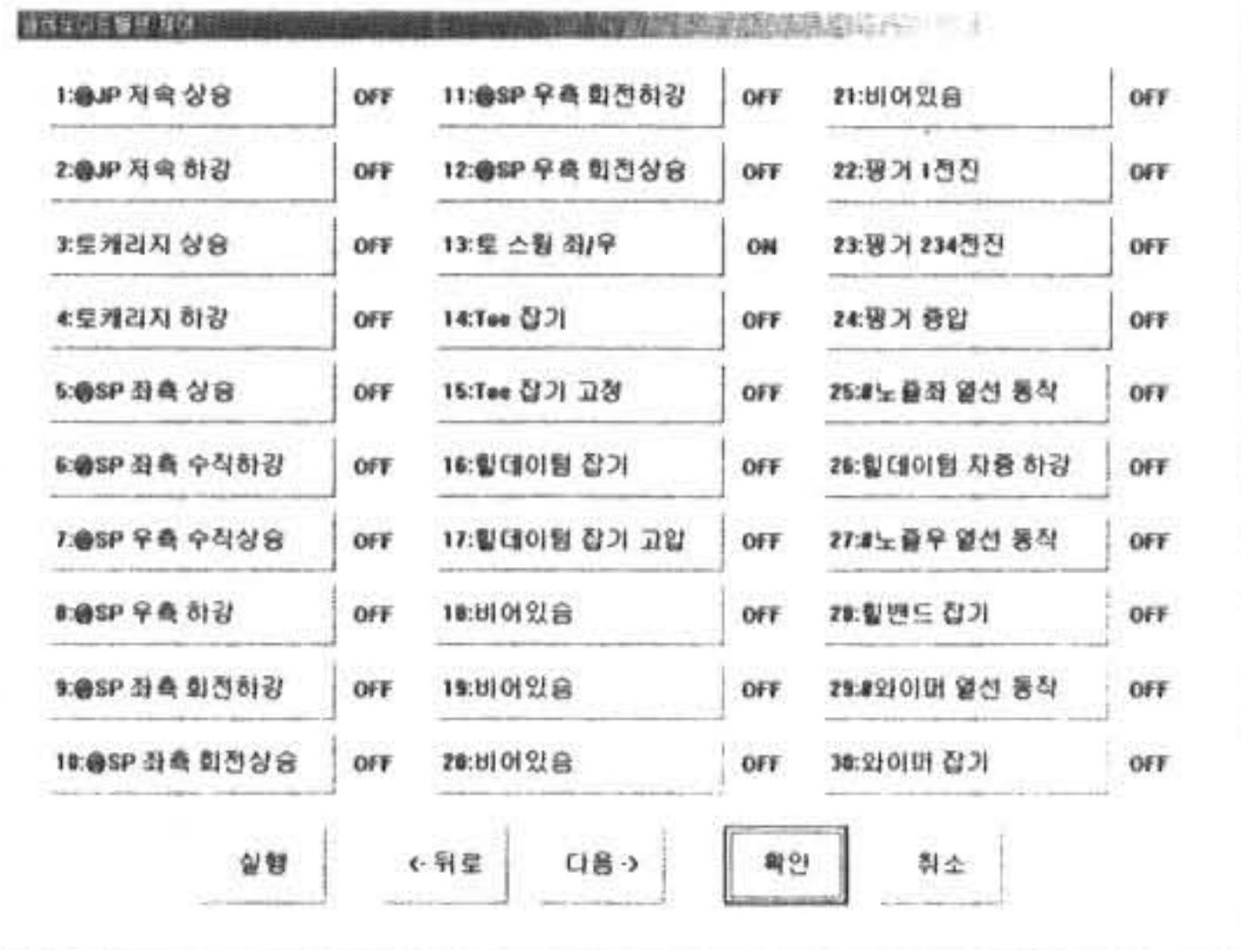
Fig. 9. Operation test window of solenoid valves
