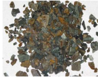
Fig. 2. Crushed coarse aggregate
