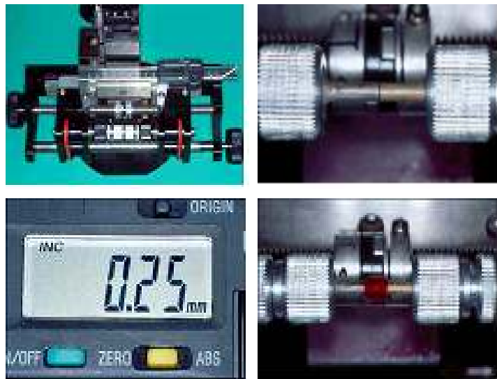
Fig. 3. Specially designed holding device was used to keep two halves of specimen with even gap.
