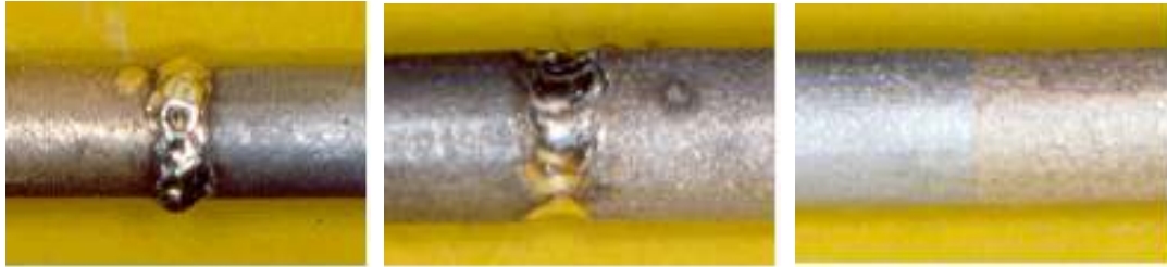
Fig. 5. All humping and spatter of laser welded or soldered specimen were carefully removed.
