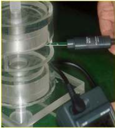
Fig. 4. The evaluation of strength of magnetic fields with gauss meter
