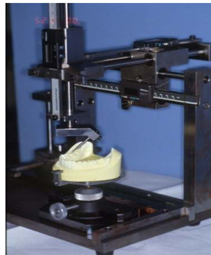
Fig. 6. The measuring points were recorded on the computer, after setting the contact point of both central incisors as reference point(0,0,0),
