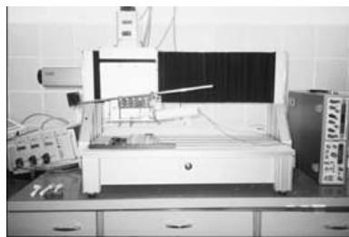
2b. Custom made brushing machine
