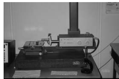
2c. Profilometer (S6P, Perthen, Hannover, Germany)
