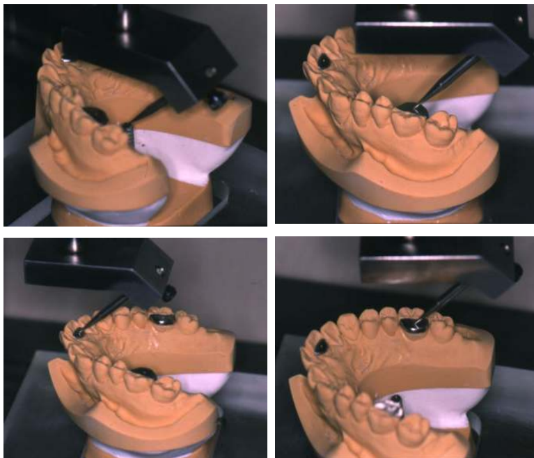
Fig. 6. Measurement of reference point and three measuring points.
