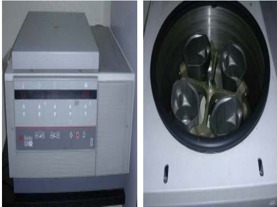
Fig. 5. IEC central GP8R centrifuge (IEC, Needham Heights, MA, USA) (left:outside view, right:inside view).
