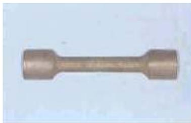
Fig. 3. Tensile specimen cast in precious metal-ceramic alloy.
