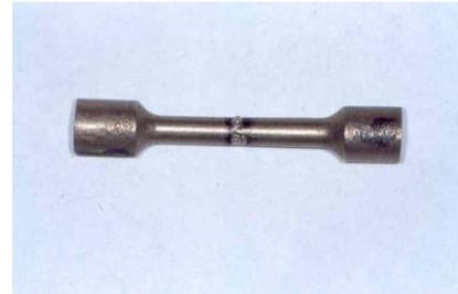
Fig. 9. A laser-welded joint exhibited a shiny silver surface. It was accepted as suitable welding quality.
