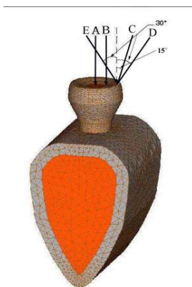
Fig. 4. Five loading direction of loading condition A, B, C, D, E.
