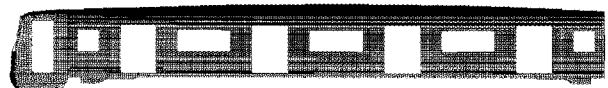
Fig. 5 1st bending mode shape of the car body in the free vibration analysis
