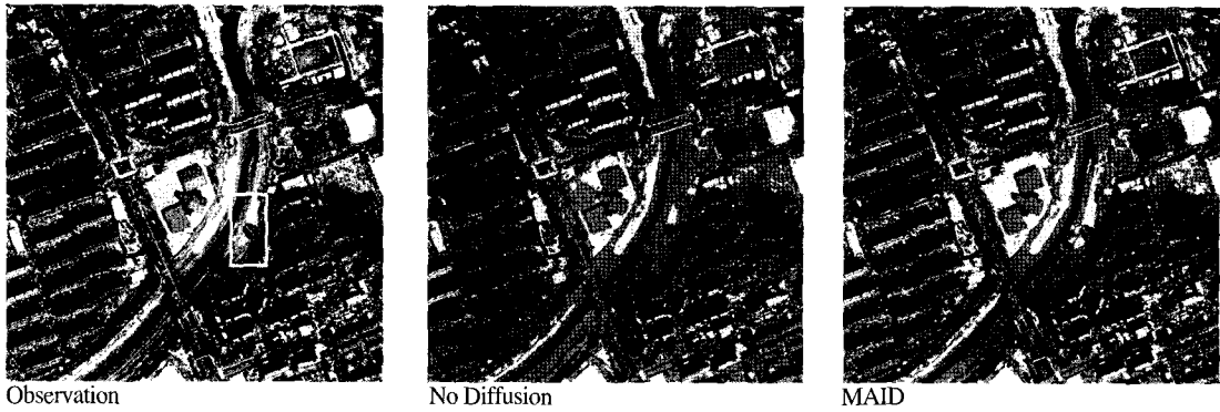
Fig. 9. Classification results of IKONOS panchromatic image observed from Gangnam area with 4 classes ( K_0 = 50 and \zeta_K = 2.0 for MAID).
