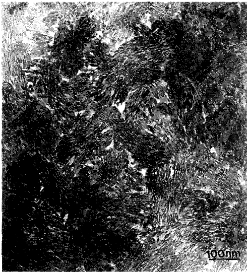
Fig. 2. Bright field transmission electron microscopy image of bulk EMD material.
