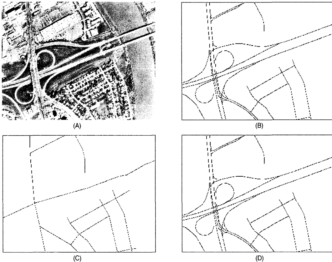
Fig. 4. Types of road features using high-resolution satellite image (Han, 2001): (A) A sample image of IKONOS 1M, (B) Double centerline, (C) Single centerline, and (D) Foot-print type.
