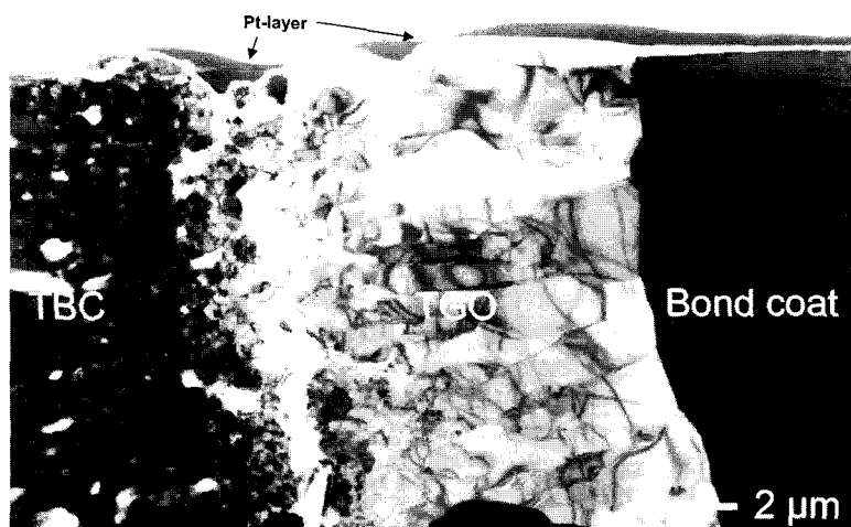
Fig. 11 Bright field TEM micrograph of intact electron beam physical vapor deposited TBC specimen after 645, 10-hour thermal cycles at 1038°C. Extensive decohesion at or near the YSZ/TGO interface was observed
