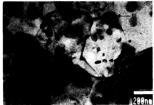
Fig. 5. Bright-field electron micrograph of Al_{73}Si_{19}Ni_7Ce_1 alloy extruded at 400°C and an extrusion ratio of 10 : 1.
