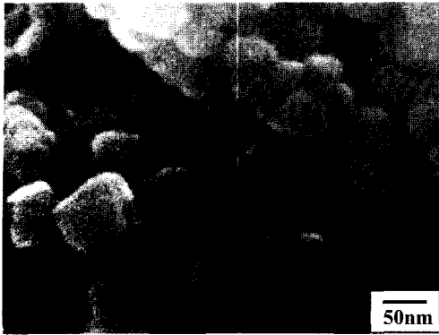
Fig. 6. SEM microstructure of nano-structured titanium carbide.
