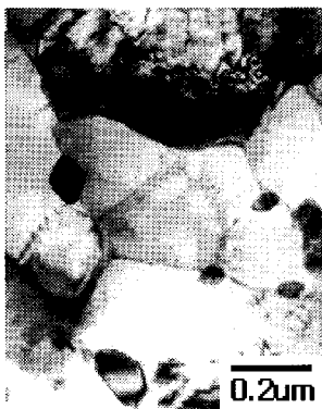
Fig. 2 TEM micrographs showing strain-free polygonal ferrite grains in the sample tempered at 973k
