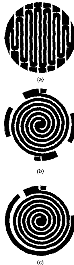
Fig. 1. The pattern shapes of current limiting elements. (a) meander shape, (b) bi-spiral shape (c) spiral shape.
