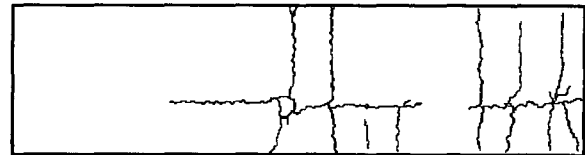
Fig. 18 Extracted crack of subway inner wall
