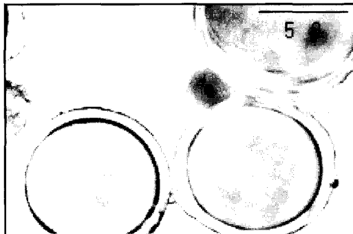
Photo 6. Optical micrograph of atactic PVA/PVAc skin/core microsphere dyed with 0.1g/100 ml of C.I. Acid Yellow 235 at 40°C for 1hr.
