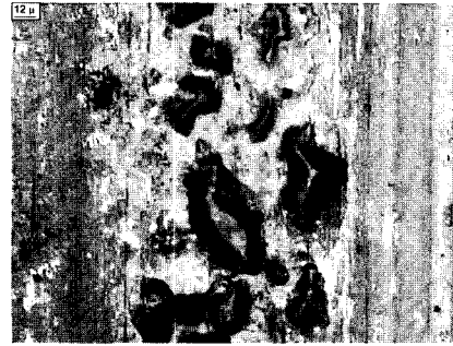
Fig. 9. The microscopic view of blisters developing in remained MoS 2 film (x200).
