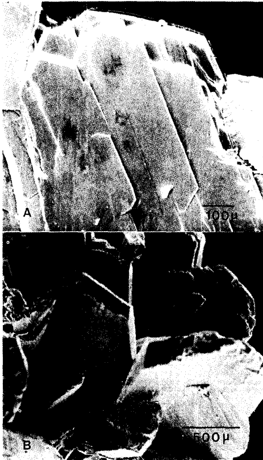
Fig. 4. SEM photographs of stilbite and stellerite. A: Common appearance of stilbite showing twinned morphology. B: Typical crystals of stellerite showing orthorhombic symmetry.
