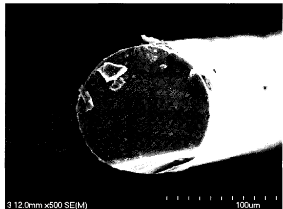
Fig. 2. FE-SEM image of a fiber heat-treated at 1300°C.
