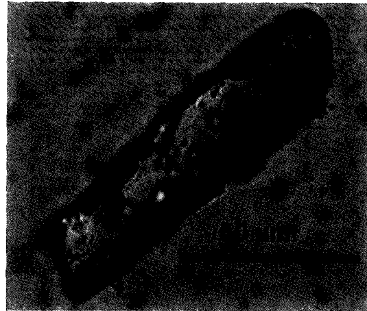
Fig. 4. Image of polished single stishovite synthesized at 15 GPa and 1400^\circ\text{C} .
