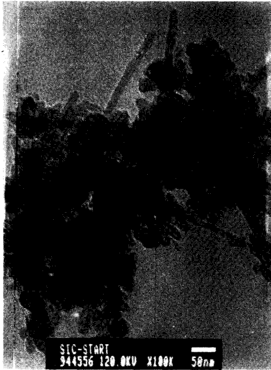
Fig. 2. Transmission electron micrograph of SiC starting powder.
