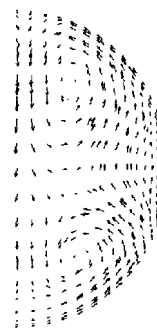
Figure 4. Velocity distribution of airflow when the throttle valve is opened to 20 degree (Maximum Vel. = 141.3 m/s): (a) at the plane y = 0 , (b) zoomed plot, (c) at the plane x = 0.3 and (d) at the plane x = 0.6 .
