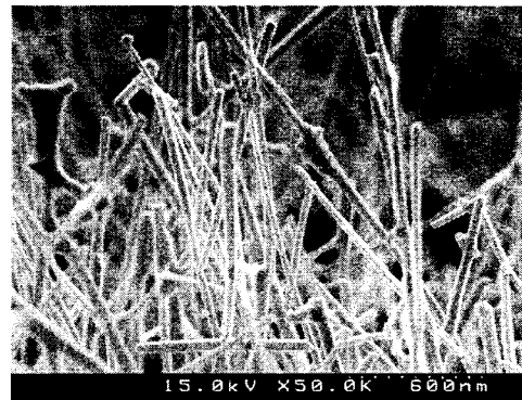
Fig. 13 50K magnified SEM image of carbon nanorods formed on a SUS304 substrate using Ni(NO 3 ) 2 (radial distance from flame axis = 5 mm)
