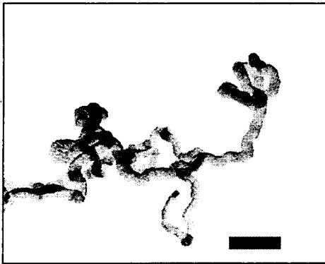
Fig. 5 TEM image of carbon nanofibers formed on a SUS304 substrate (length of scale bar = 200 nm)
