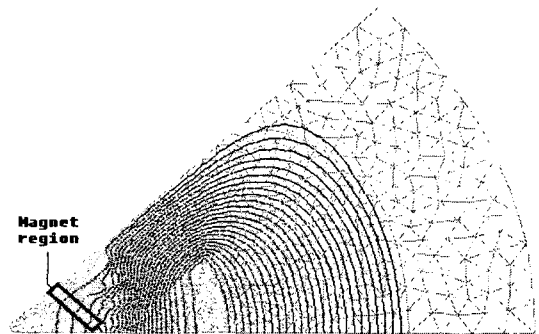
(b) Magnetic flux distribution at t_1 (when the slope of current is large)
