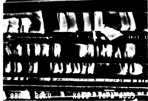
Fig. 12 Fracture surface of ENF specimen in dynamic test(CU125NS [0^\circ_{20}] )
