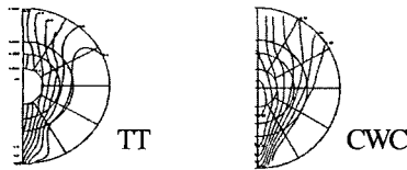
Fig. 13 Wake measurements at F_n=0.266 (Series 60, C_b=0.6 )
