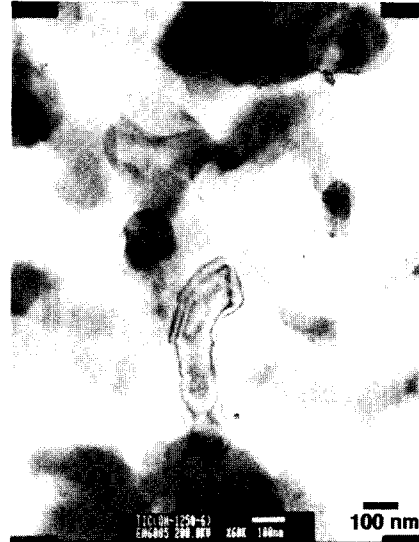
Fig. 13. TEM microstructure of TiC-15%Co powder reduced/carburized at 1250°C for 6 hours in H 2 .
