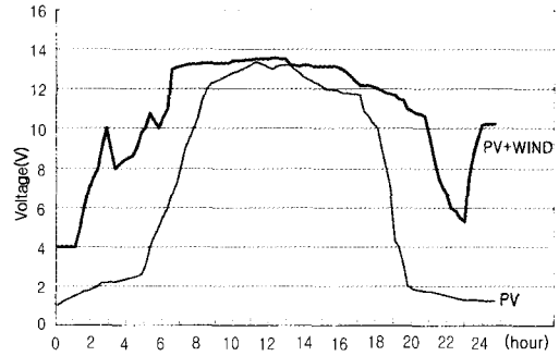
Fig. 10 Voltage characteristics of the PV and wind turbine
