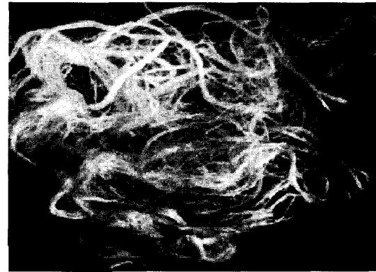
Fig. 9. 105 DAP Kenaf bast fiber bundles after chemical retting with 7% NaOH
