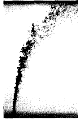
(a) 1.0 round edged orifice at 3 bar( q=82.49 )
