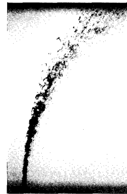
(c) 1.0 sharp edged orifice( L/d=5 ) at 4 bar( q=71.43 )
