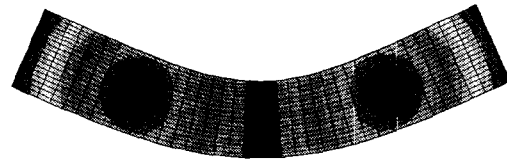
Fig. 2 Typical result of finite element analysis for the uniform beam model with a crack at the mid span
