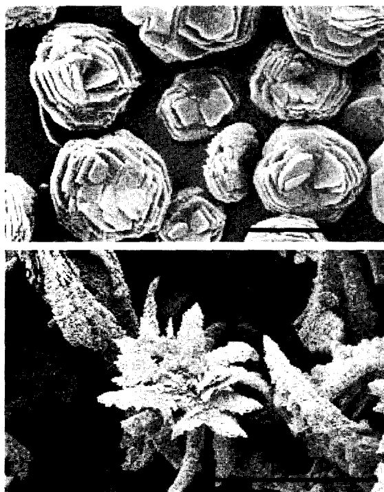
Fig. 1. (a) Calcium oxalate formed by solubilization of apatite ( \text{Ca}_5(\text{PO}_4)_3\text{OH} ) and (b) lead oxalate formed by solubilization of the lead-containing mineral pyromorphite ( \text{Pb}_5(\text{PO}_4)_3\text{Cl} ) by Serpula himantiooides .
