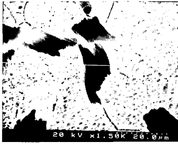
Fig. 13 SEM line profile after immersion test in 35%HCl during 96 hours for Dis1300
