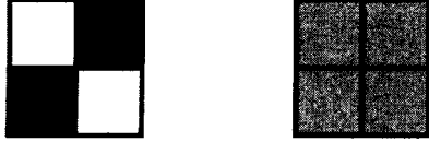
(a) Checkerboard pattern (b) Uniform density pattern Fig. 7 Material distribution
