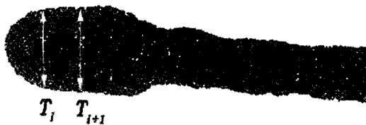
Fig. 5. Definition of the width variation between head and tail of a liquid track
